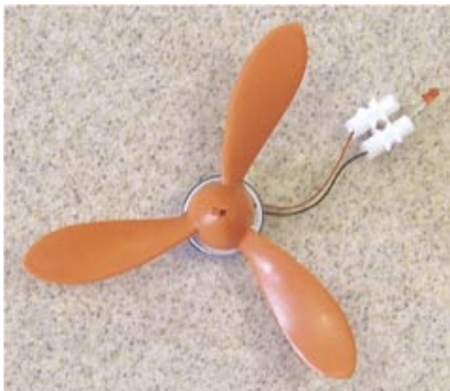
Figure 9 - Model turbine (propellor, terminal block & red LED)
