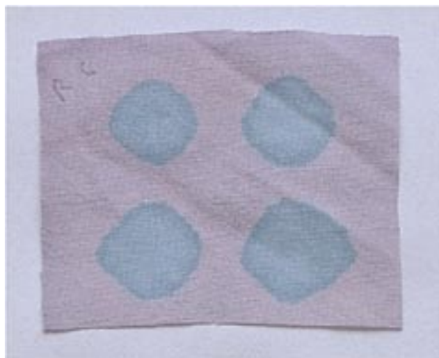
Figure 7 - Fabric stained with red cabbage vinegar. Drops of alkali added.
