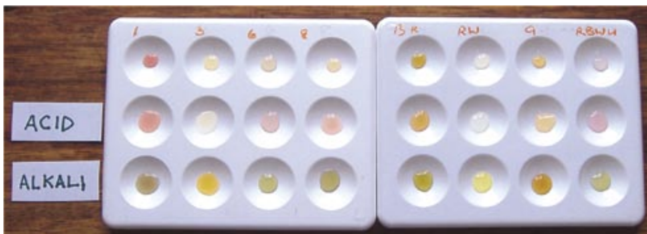
Figure 5 - Top row - Plant extracts, Middle row – Drop of vinegar added, Bottom row - drop of sodium bicarbonate added
