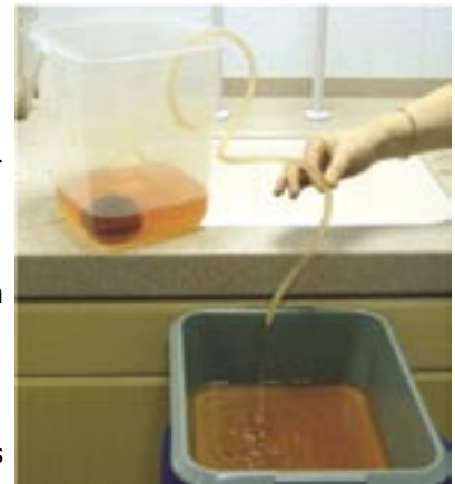
Figure 14 - Syphon at work.
